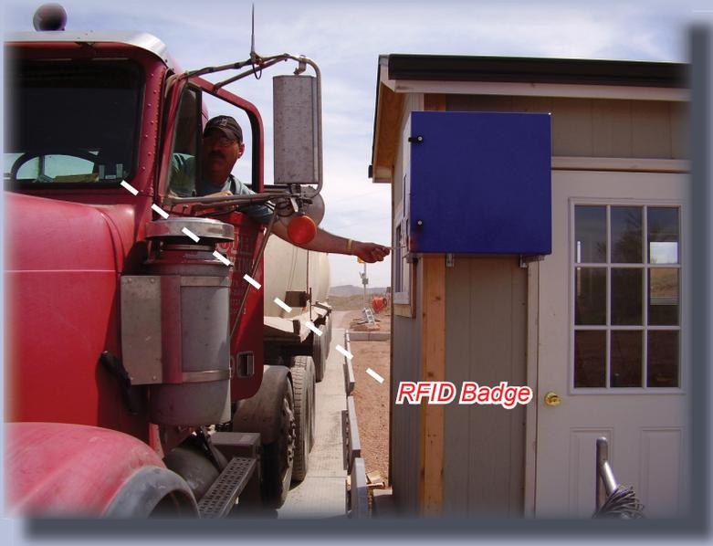
Both Remote Printers are driver-friendly. The ticket can be processed manually by the scale attendant or automatically in cases where Jobs/Orders can be dispatched through Interact® software to each truck prior to the transaction taking place. (Options such as RFID readers are available to identify the truck on the scale.) In either case, once the information is entered into the software, the driver receives their ticket without ever leaving the truck!
