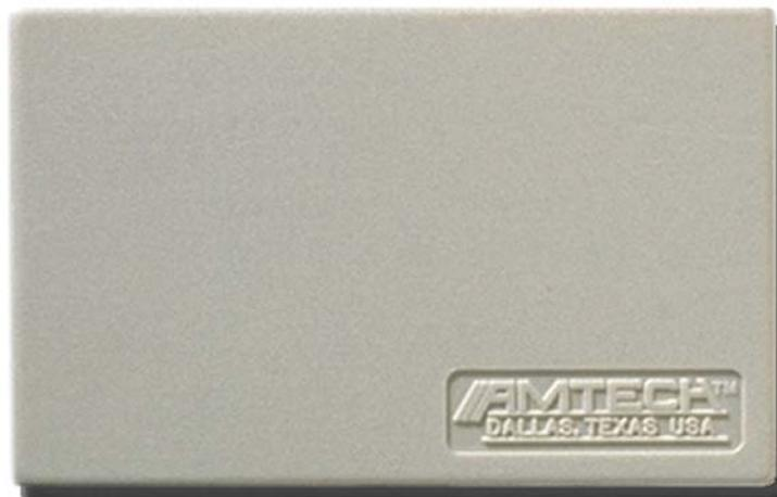
The AT5402 Access Control Tag is a half frame, beam-powered radio frequency (RF) tag used in automatic vehicle identifications with TransCore's Amtech-brand and TransCore Encompass multiprotocol reader systems. This tag is designed for interior mounting on a nonmetallized windshield.
